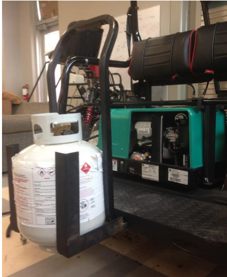
Figure 2. Photograph of the propane tank mount.
